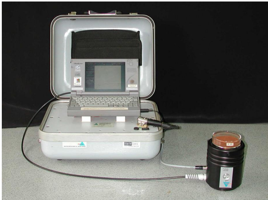
Fig. 1. Field portable spectrometer showing the optical set up.
